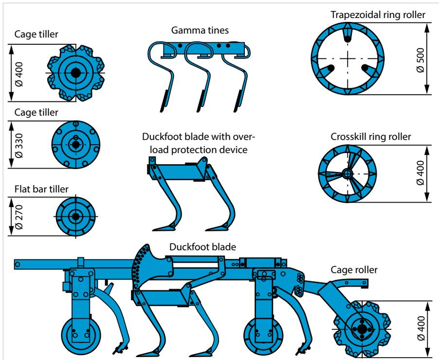
The System Kompaktor is available with many combination options. Next to the various tine sections, cage tilling rollers or flat bar tilling rollers can be combined with various following rollers. This effectively means that the System Kompaktor is an implement suitable for use in almost any soil conditions.
