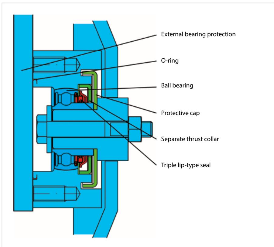
The new generation of maintenance-free bearings has been completely sealed thereby effectively protecting it against any soiling. This guarantees a high service life.
