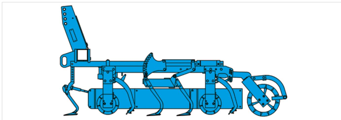
The System Kompaktor frequently achieves the required working quality in only a single pass.
