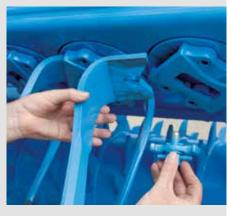
Replacing a quick-change tine
