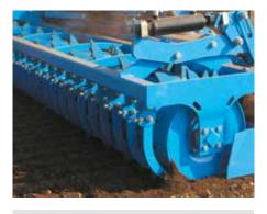
Tooth packer roller for medium and heavy soil conditions
