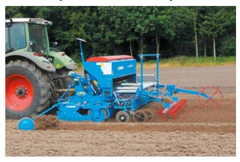
It is becoming ever more important to adjust the intensity of the seedbed preparation to the prevailing field conditions. Practice shows that the power harrow is a very versatile and efficient device and therefore best performs this preparatory task.
