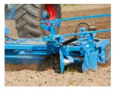
Feed discs for precisely harrowed paths
