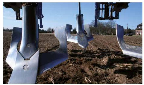
The Kristall compact cultivator from LEMKEN can be used for both shallow and medium depth work in several stages. The initial shallow cultivation involves the specially shaped TriMix stubble shares working volunteer grain and organic mass into the soil across the entire width and close to the soil surface. The volunteer grain remains in the upper layer of soil where it will quickly germinate.
